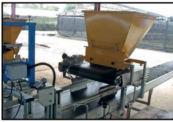
hopper is fitted with adjustable sides
