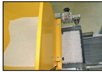
substrate hopper is mounted over the feeding belt
