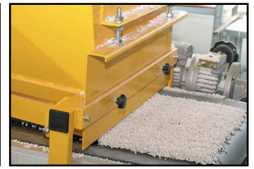
adjustable gate to determine thickness
